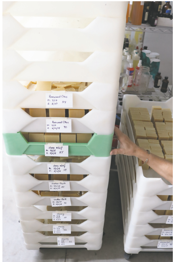
After production, soaps are organized by scent and kept in a cool, dry environment before they are packaged.
